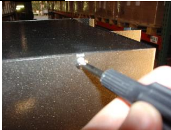
Remove top cover on tower mast
